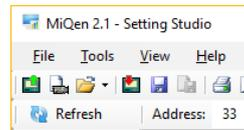
Factory default Modbus address for all devices is 33. Therefore it is required to change Modbus address number of devices if they are connected in the network so each device will have its unique address number.
