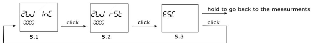
Holding button on screen 5.1 include or exclude ZWave from network. Holding button on screen 5.2 resets ZWave module.
