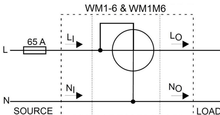
Figure 3: Electrical diagram 230 V<sub>AC</sub>
