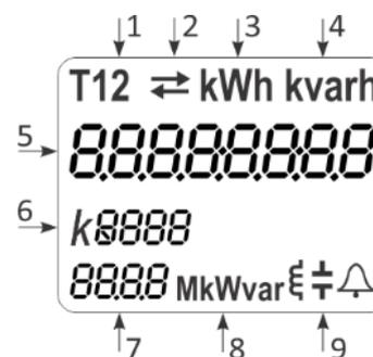
**Figure 8:** Layout of LCD
