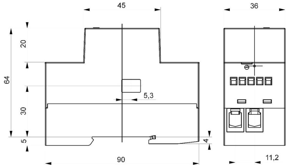
**Figure 2:** Dimensional drawing and rear connection terminals position
