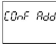
During this time, the WM1-6A responds to the 149 address via the ModBus. The device remains in configuration mode until the ModBus address is modified or when 3 minutes pass or with a long press of 1 second to 3 seconds.
