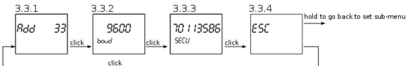
Screens 3.3.1 shows the primary address of M-bus communication, screen 3.3.2 shows baud rate and screen 3.3.3 shows the secondary address.
