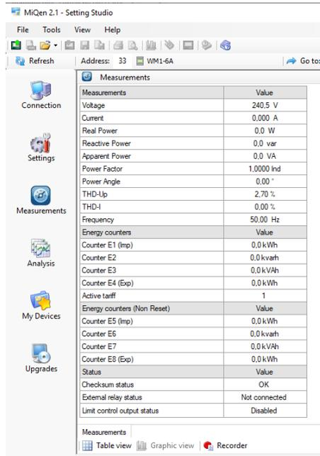
The screenshot shows the 'Measurements' section of the MiQen 2.1 software. The interface includes a menu bar (File, Tools, View, Help), a toolbar with icons for refresh and address, and a sidebar with navigation options (Connection, Settings, Measurements, Analysis, My Devices, Upgrades). The main area displays a table of measurements with columns for 'Measurements' and 'Value'.
