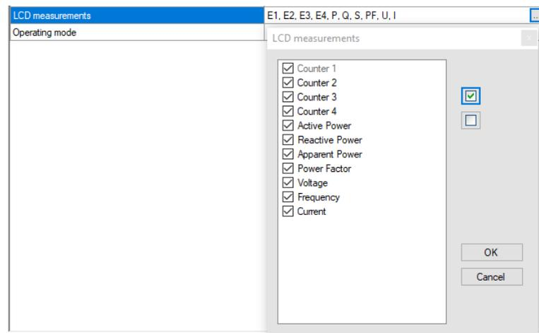
**Figure 12:** Set of optional measurements
