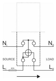
Figure 1: Connection diagram
