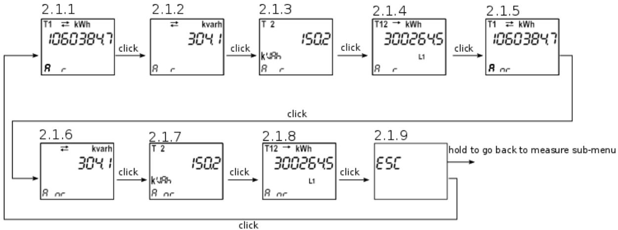
Holding button on any of screens 2.1.1 through 2.1.8 sets this screen as a meter screen.
