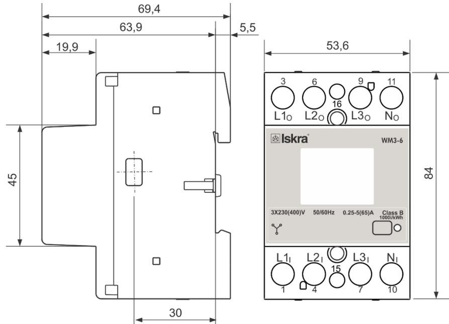
**Figure 2:** Dimensional drawing and rear connection terminals position
