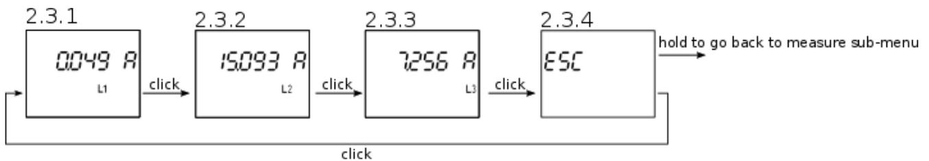
Holding button on any of screens 2.3.1 through 2.3.3 sets this screen as a meter screen.
