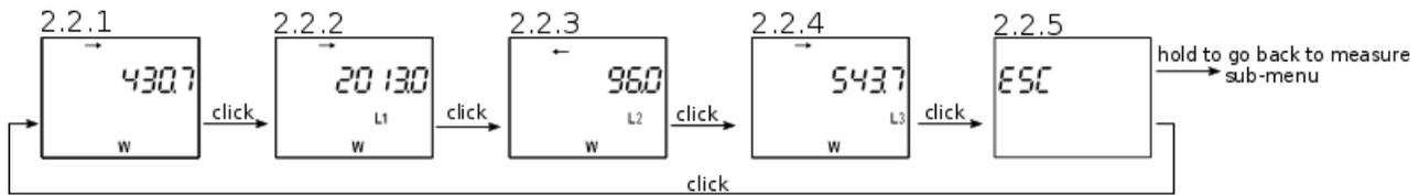
Holding button on any of screens 2.2.1 through 2.2.4 sets this screen as a meter screen.
