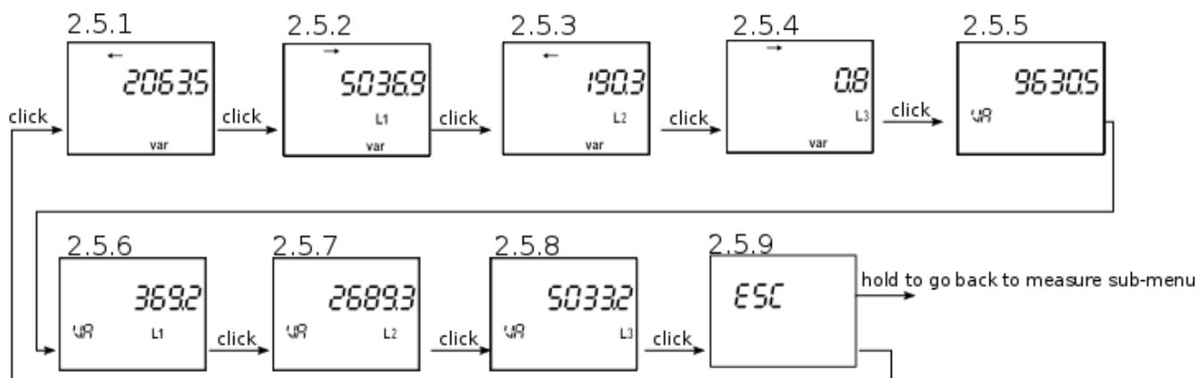
Holding button on any of screens 2.5.1 through 2.5.8 sets this screen as a meter screen.
