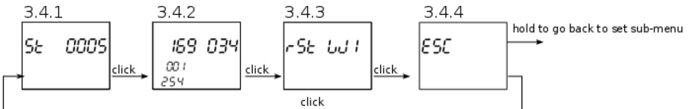
Screen 3.4.1 shows Wi-Fi status, screen 3.4.2 shows IP address of gateway module and screen 3.4.3 resets the Wi-Fi.
