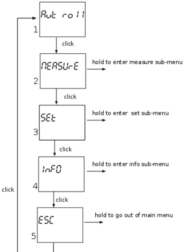
By holding the button when positioned on certain screen ( e.g. measure, set, etc...) the sub-menu is entered.
