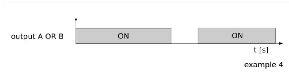
Below graphical representation of both output A AND B as well as output A OR B.
