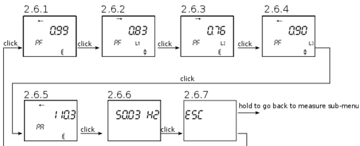
Holding button on any of screens 2.6.1 through 2.6.6 sets this screen as a meter screen.
