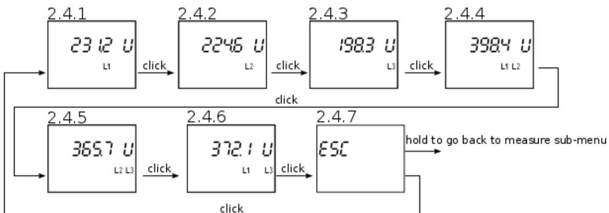
Holding button on any of screens 2.4.1 through 2.4.6 sets this screen as a meter screen.
