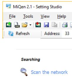
Factory default Modbus address for all devices is 33. Therefore it is required to change Modbus address number of devices if they are connected in the network so each device will have its unique address number.
