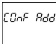
During this time, the WM3-6 responds to the 149 address via the ModBus. The device remains in configuration mode until the ModBus address is modified or when 3 minutes pass or with a long press of 1 second to 3 seconds.
