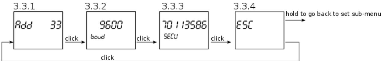
Screens 3.3.1 shows the primary address of M-bus communication, screen 3.3.2 shows baud rate and screen 3.3.3 shows the secondary address.
