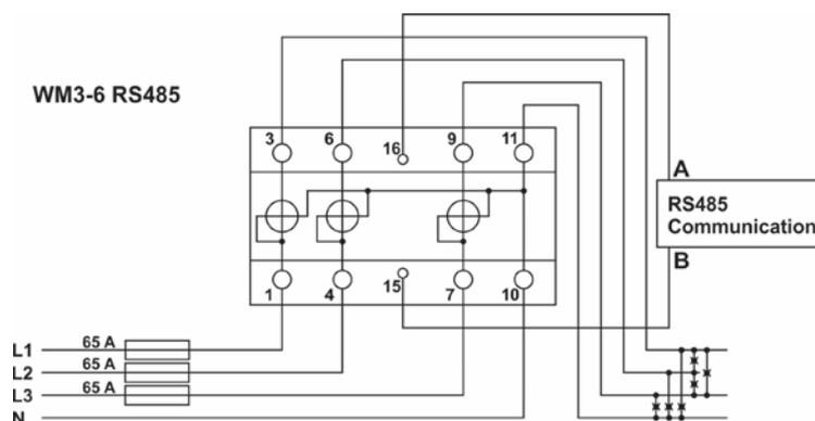
Complete WM3x6 system is assembled with three main units and optionally communication unit:
