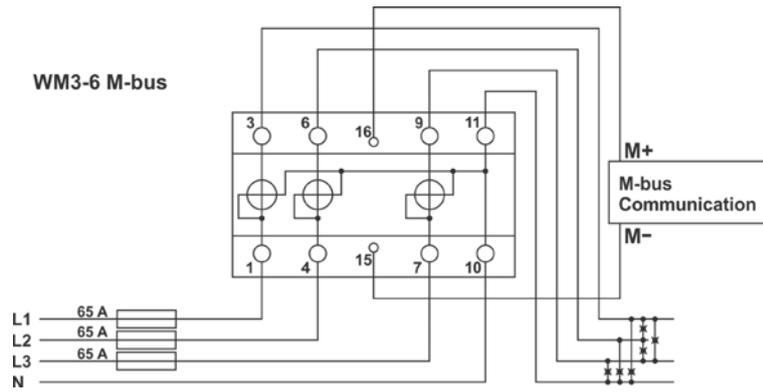
**Figure 5:** Connection diagram for pulse output option
