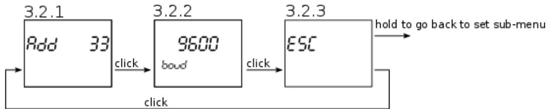
Screen 3.2.1 shows the address of RS 485 communication and screen 3.2.2 shows the baud rate.
