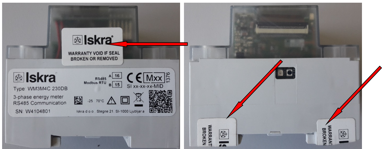
Figure 7: Location of sealing in the form of label (WM3M4C and WM3M4).
