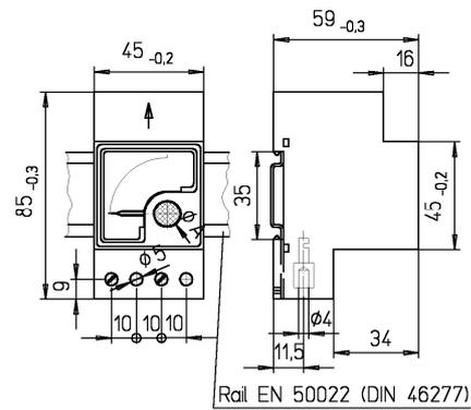
Picture 4: Dimensional drawing BQ0507 (all dimensions are in mm)
