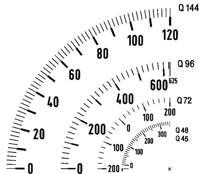
Picture 1: Drawing of scale: BQ0107, BQ0207, BQ0307, BQ0407, BQ0507 (voltmeters, ammeters)
