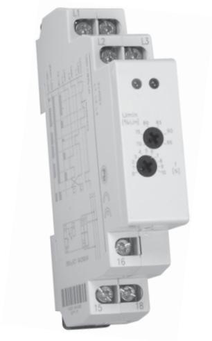
MVR 56 – RELAY MONITORS PHASE SEQUENCE AND FAILURE (E.G. CONTROL OF CORRECT MOTOR WINDING ETC.).
