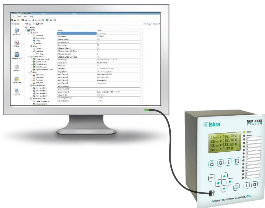
Figure 4.43 Connection between FPC device front port and PC via USB male - A to male - A.
