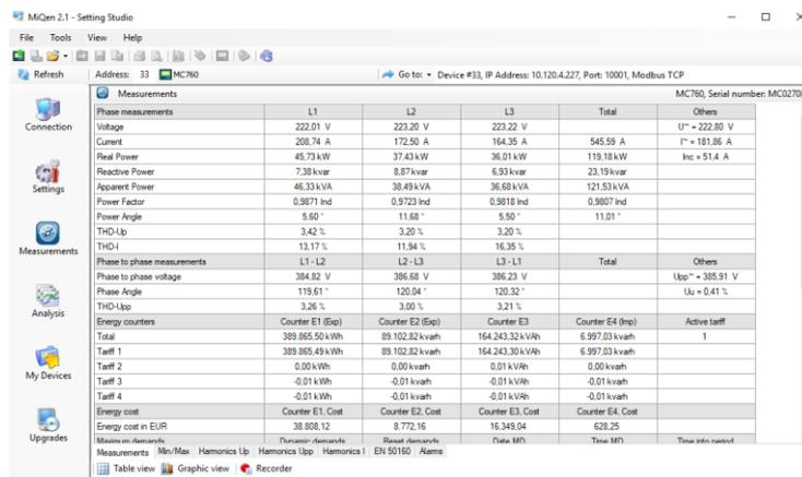
Figure 3 Sample of online measurements in tabular form
