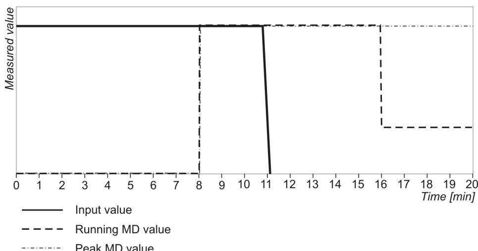
**Figure 10:** Operation of Fixed window MD function
