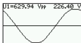
Display of a Phase Voltage in time space diagram. Displayed are also peak value of monitored phase voltage and its RMS value. Similar display is also for phase-to-phase voltages.
