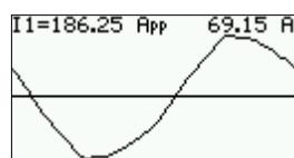
Display of a Current in time space diagram. Displayed are also peak value of monitored current and its RMS value.
