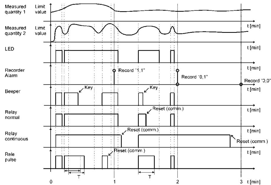
**Figure 18:** Graphical presentation of alarms operation
