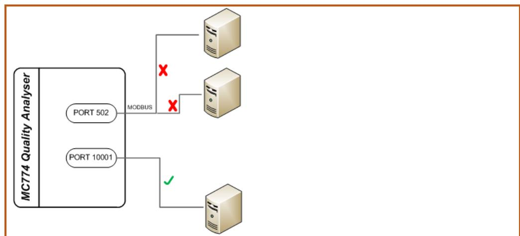
**Figure 13:** When any other allowed port is used only a single connection is possible
