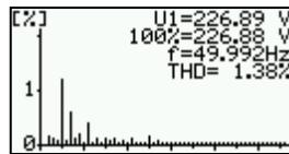
Display of a Phase Voltage in frequency space diagram. Displayed are also RMS value, unit value (100%), system frequency and THD value. Similar display is also for phase-to-phase voltages.
