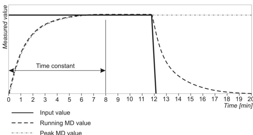
**Figure 9: Operation of thermal MD function**
