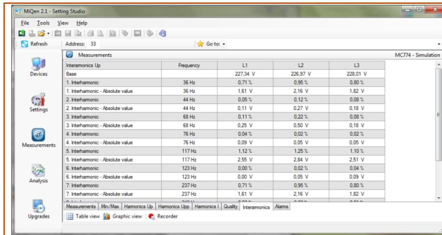
**Figure 36:** Tabularic presentation of 10 phase voltage interharmonic components
