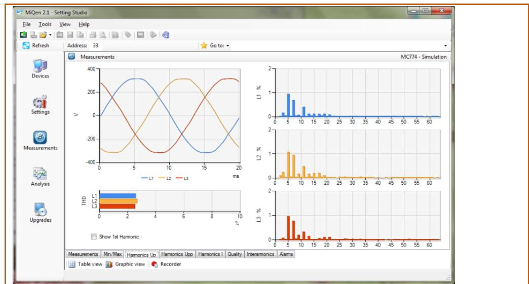
**Figure 35:** Graphical presentation of phase voltage harmonic components
