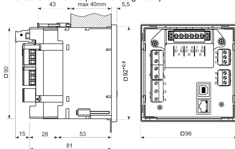
**Figure 2:** Dimensional drawing and rear connection terminals position
