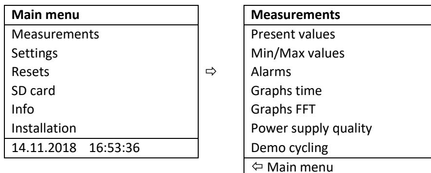
Alarms are important feature for notifying exceeded user predefined values. Not only for visualisation and recording certain events with exact time stamp. Alarms can be connected to digital/alarm outputs to trigger different processes (switch closures, line breaking, motors start or stop ...).
