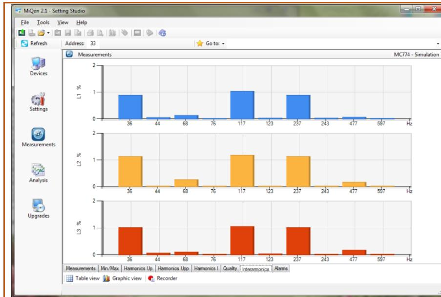
**Figure 37:** Graphical presentation of phase voltage interharmonic component
