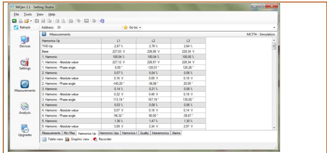
**Figure 34:** Tabular presentation of phase voltage harmonic components
