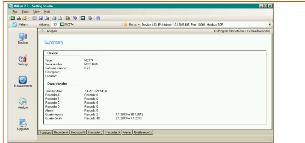
**Figure 40:** Information about downloaded data with tabs for different memory partitions
