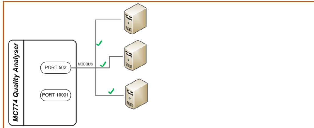
**Figure 12:** Multiple connections to a device are possible when port 502 (special MODBUS port) is used
