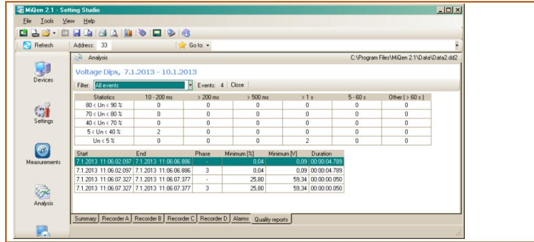
**Figure 46:** Presentation of Dips and Interruptions in a list (only four events) and in a statistics table
