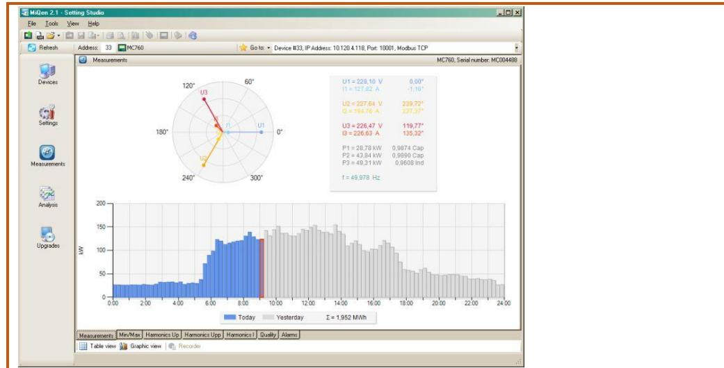
**Figure 26:** Online measurements in graphical form – phaser diagram and daily total active power consumption histogram
