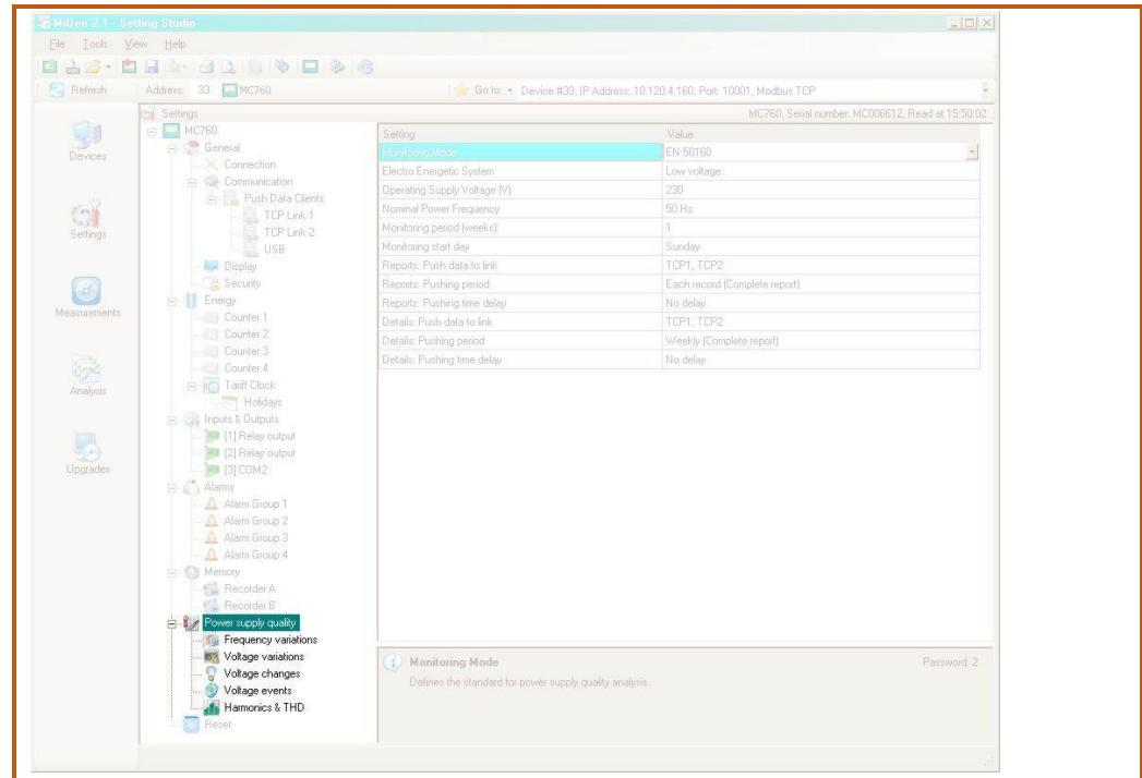
**Figure 24:** Settings for power quality parameters are set with setting and monitoring software MiQen
