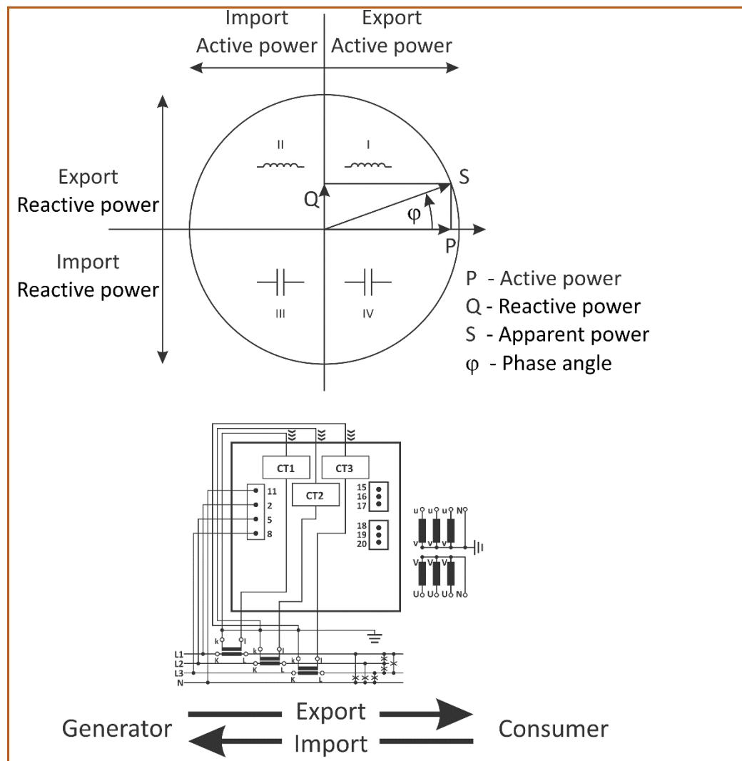
Figure 29: Explanation of energy flow direction
