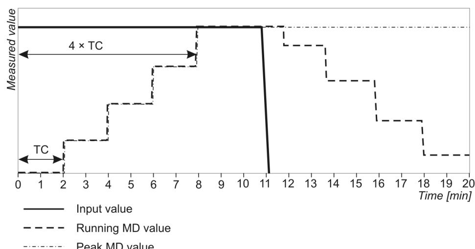
***Figure 11: Operation of Sliding window MD function***
