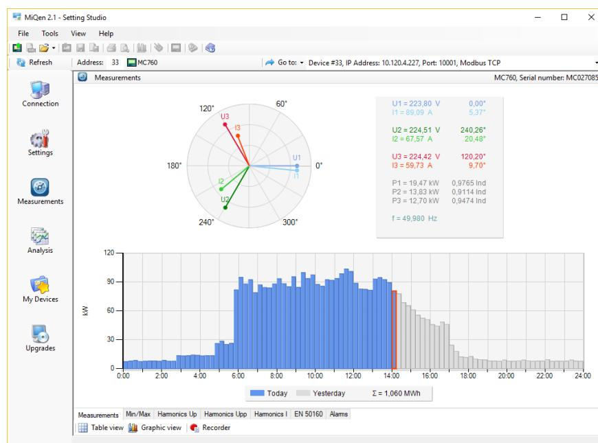
Figure 6: Online measurements in graphical form – phaser diagram and daily total active power consumption histogram.
