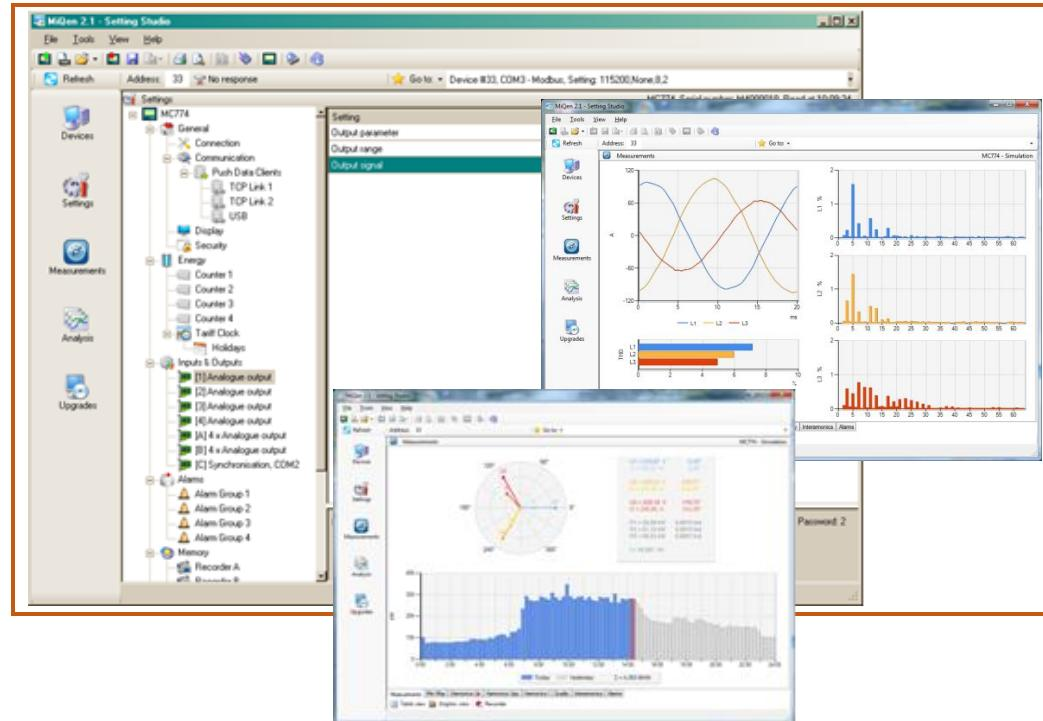
MiQen version 2.0 or higher is required for programming and monitoring MC 7x0A Power Monitoring Device. Software installation can be downloaded from [www.iskra.eu](http://www.iskra.eu).
