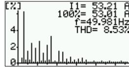
Display of a Current in frequency space diagram. Displayed are also RMS value, unit value (100%), system frequency and THD value.
