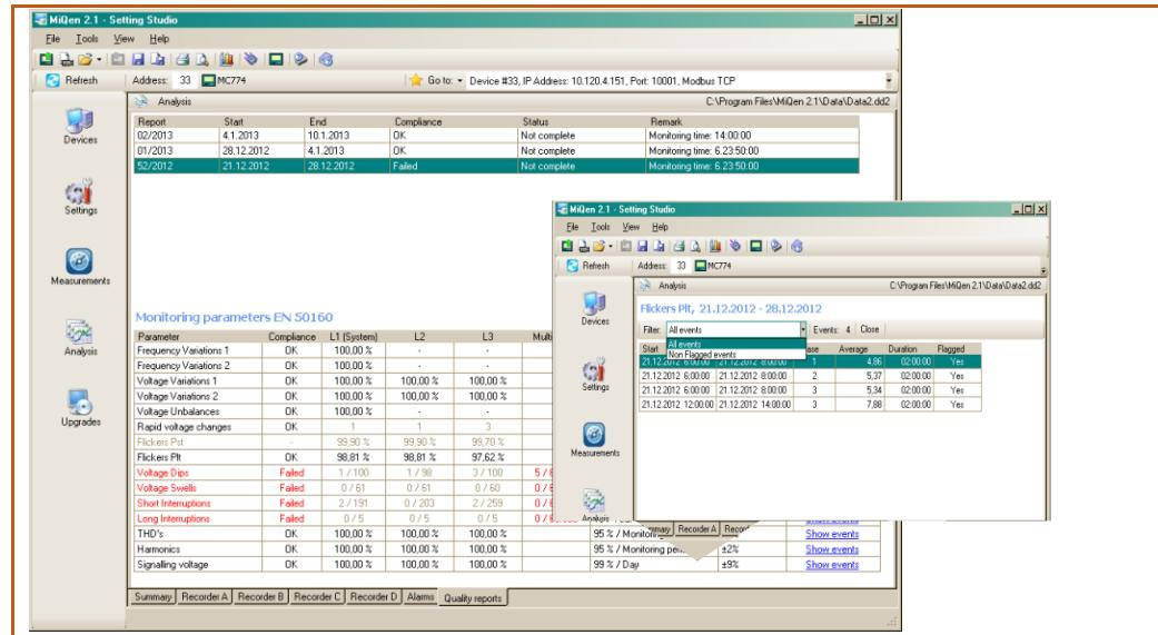
**Figure 42:** By clicking on “Show details” for each PQ parameter MiQen displays time-stamped measurements (events), which were outside limit lines
