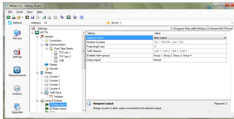
**Figure 15:** MiQen window for digital output definition
