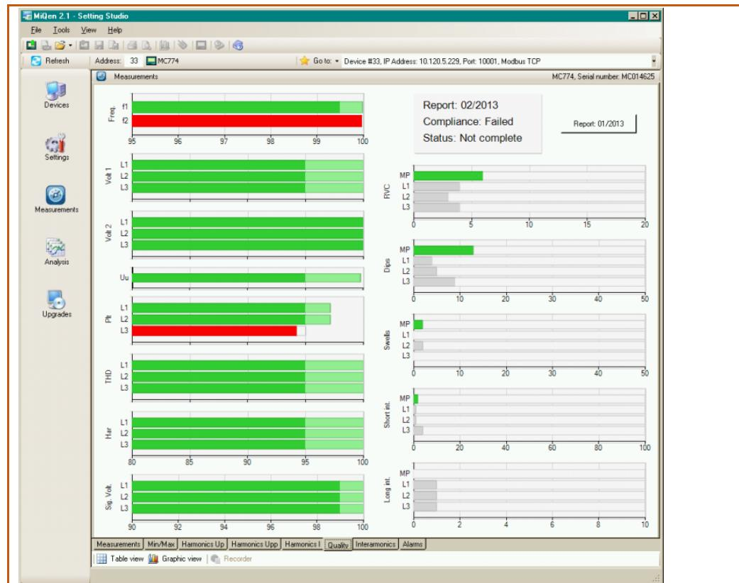
**Figure 39:** Graphical presentation of PQ parameters and overall compliance are available only for actual monitoring period
