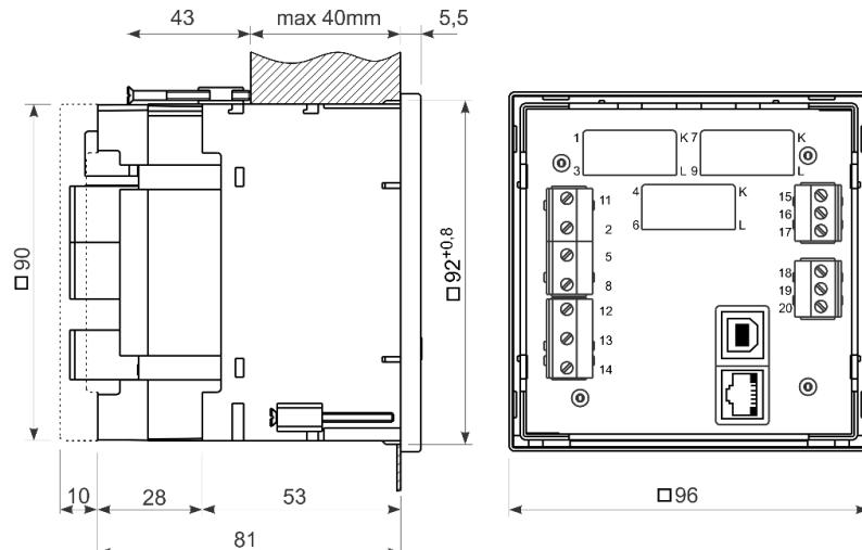
Dimensions for MC 7x0 (terminal assignment):
