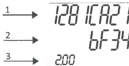
Figure 2: WM3M4C/WM3M4 example of FW identification
