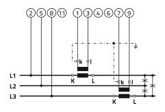
4b - three-phase, four wires, balanced load
