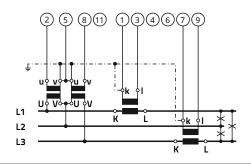
3u - three-phase, three wires, direct connection
