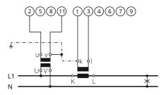
3b - three-phase, three wires, balanced load
