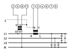
4u - three-phase, four wires, unbalanced load
