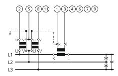
3u - three-phase, three wires, unbalanced load
