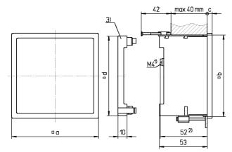
Picture 4: Dimensional drawing BQ2107, BQ2207, BQ2307 and BQ2407 (all dimensions are in mm)
