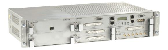
SparkLight HSP is a compact, powerful, user-friendly and easy to install device for providing transmission of PDH (E1, E3) and Ethernet over optical fibers, that enables service providers to offer subscribers reliable, high-performance, high-speed communications services such as LAN interconnection, Internet access, voice & data services, etc.
