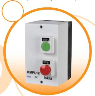
They are mainly used for start-up, overload protection and switch-off of electric motors and also for other loads. A contactor and a corresponding bimetal relay are built in the enclosure of degree of protection IP55. They are switched on with the ON pushbutton and switched off with the OFF pushbutton. The mushroom pushbutton functions as an emergency stop pushbutton.
