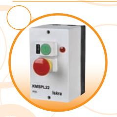
They are mainly used for start-up and switch-off of electric motors up to 11 kW power. MS25 motor protection switch with undervoltage release and a corresponding contactor are built in the enclosure of degree of protection IP55.
